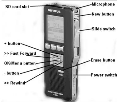
1. Turn on your Olympus DS-5000 by sliding the power switch on the lower right side of the recorder to **ON**.
