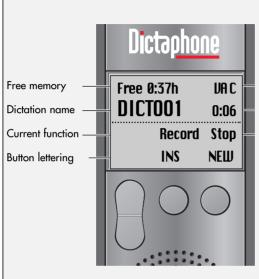
Battery symbol for low battery/rechargeable battery. Indication for voice activation and microfone sensitivity Dictation position, total length Slide-switch position
