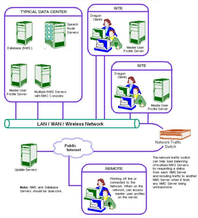
Notice that a Master User Profile Server local to the client provides rapid access to user profiles.
